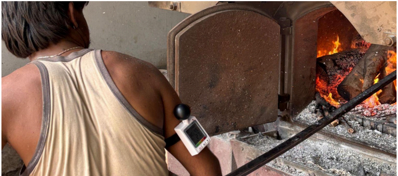
Image 11: WBGT Sensor on a Worker in the Boiler Area
